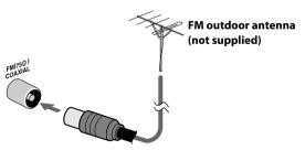
Disconnect the supplied FM antenna, and connect to an outdoor FM antenna using a 75  $\Omega$  wire with coaxial type connector.
